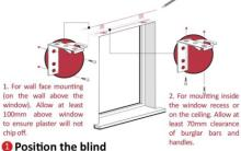
Hold the blind in place where you are going to install it, making sure that it is centered and level. When positioned correctly, mark the position of each ladder lace that supports the slats onto the wall/surface with a pencil. Position each bracket approximately 45mm to the left or right of the pencil marks and then mark the position of the bracket holes onto the wall/surface with the pencil. Ensure that the brackets do not block the tilting mechanism.
